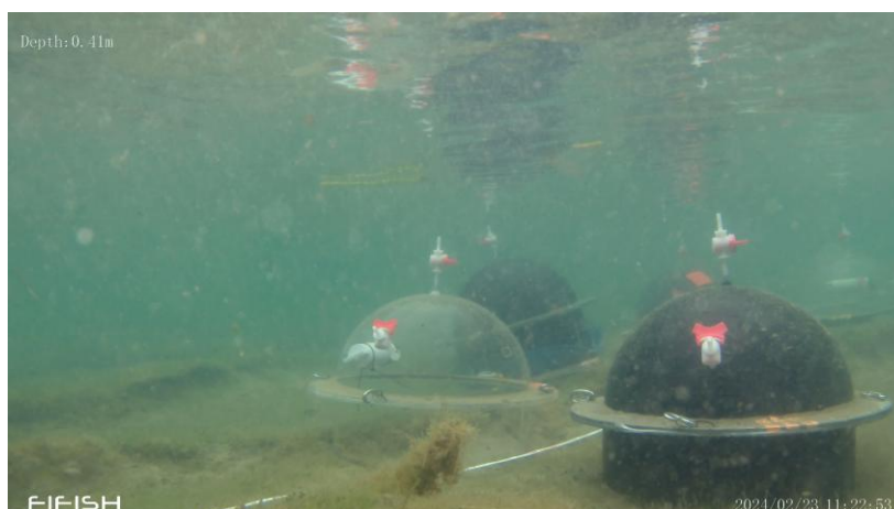
Figure 2: example of benthic chamber set up for measuring fluxes across the sediment-water interface
